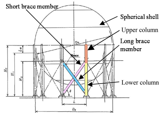
Fig. Spherical Tank with steel pipe brace and column structure
