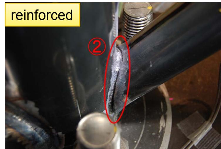
Broken brace around weld joint with lower column
