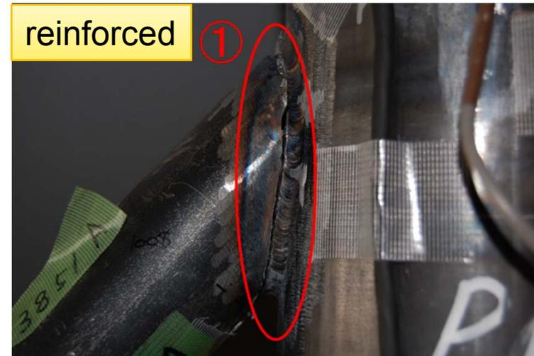
Broken brace around weld joint with upper column
