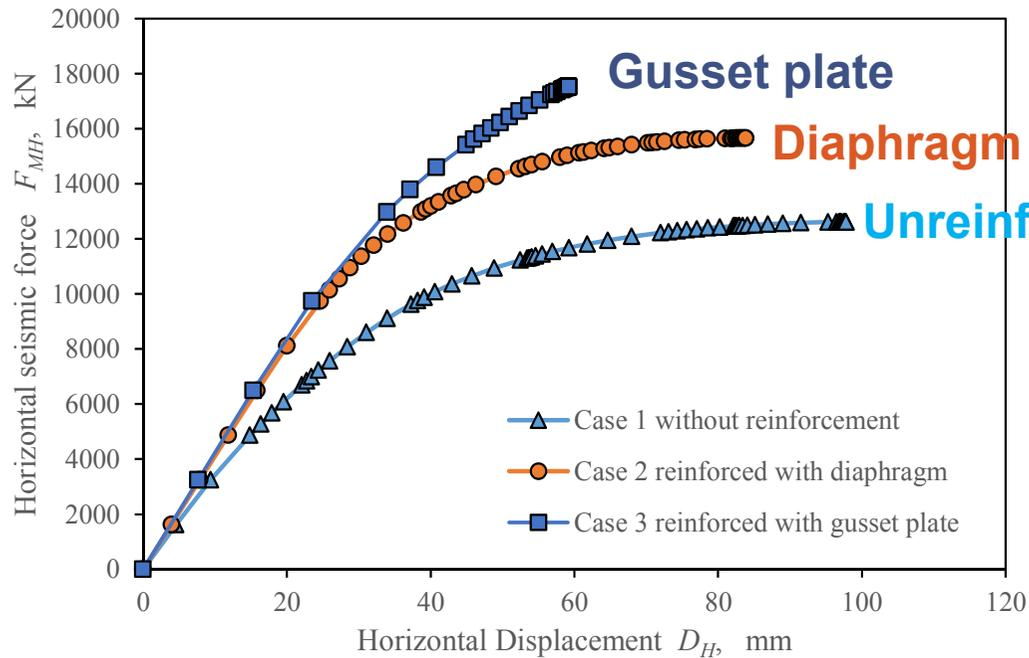
Fig. Relationship of Force and displacement
