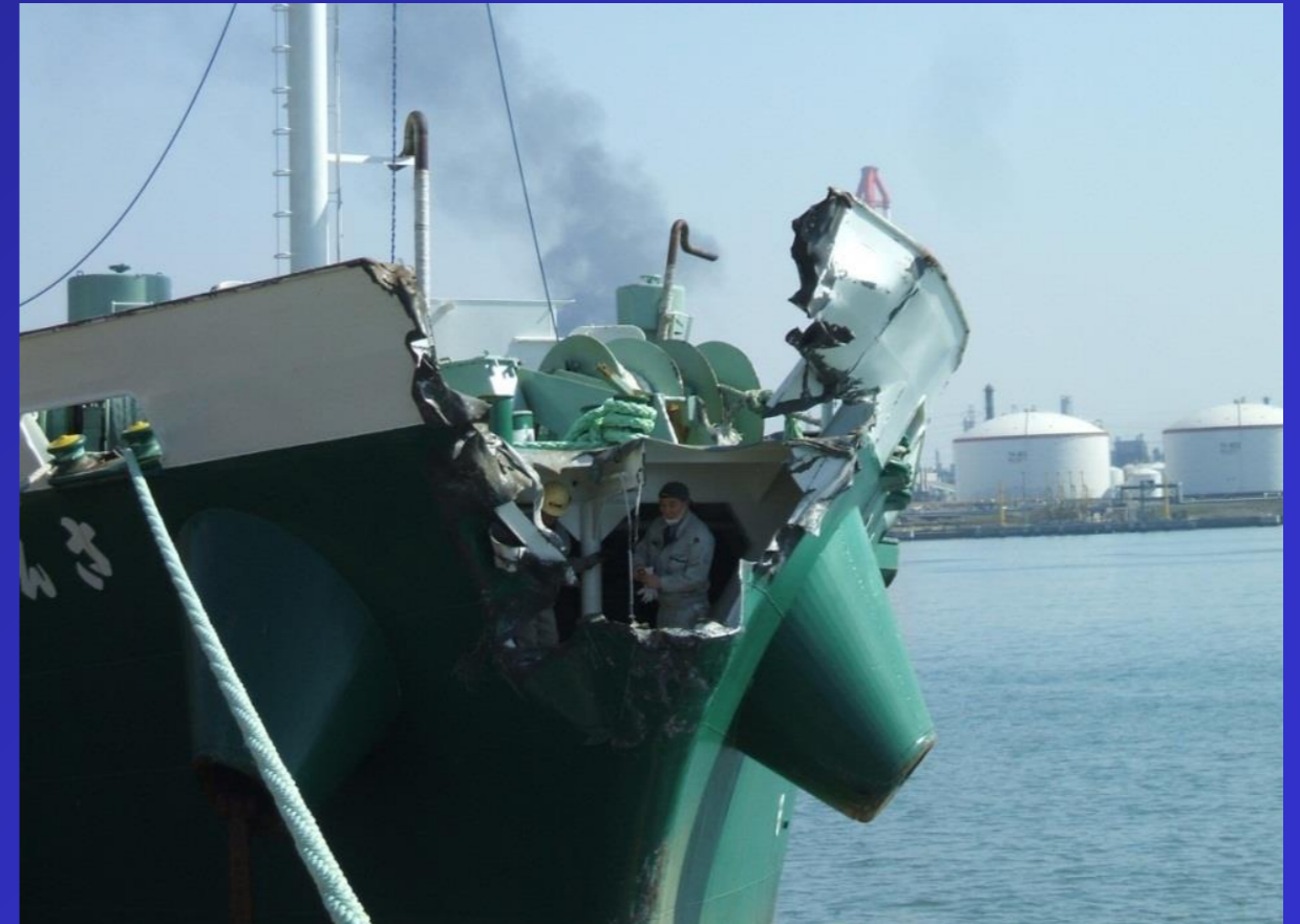
Torn off the bow by large vessel of the anchor chain
