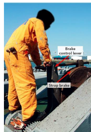
Fig. 3 Simulated position of the Seaman on the electric motor of the starboard side anchor winch (9)
