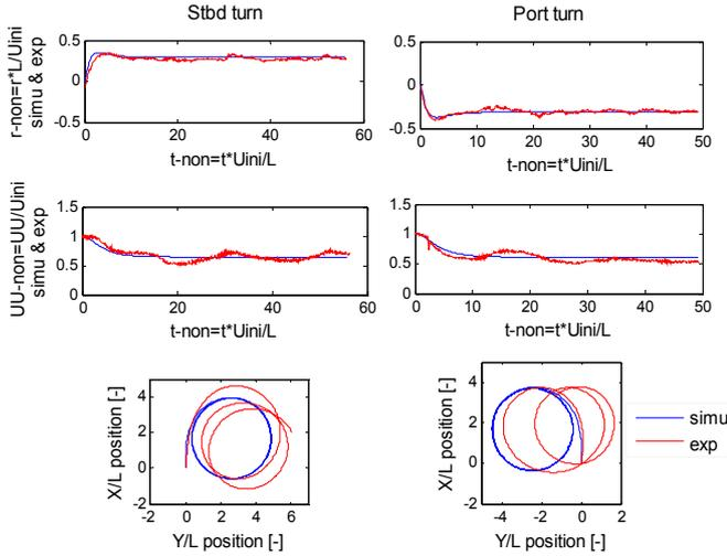
Fig. 2(b). Turning circle compassion for  $\pm 20^\circ$
