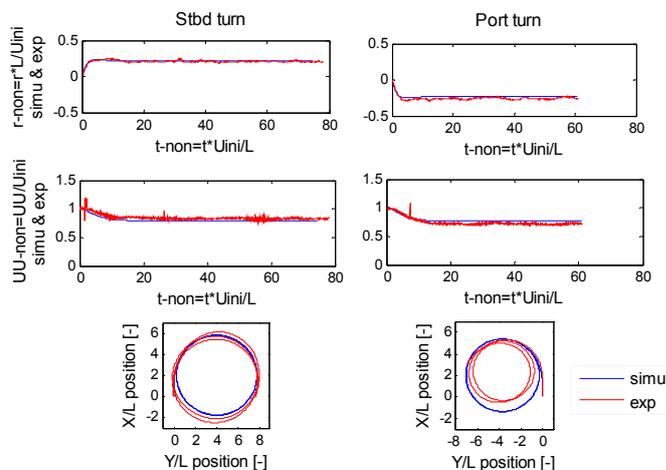
Fig. 2(a). Turning circle comparison for  $\pm 10^\circ$
