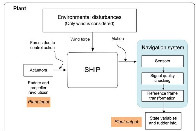
Fig. 7. Plant to be controlled
