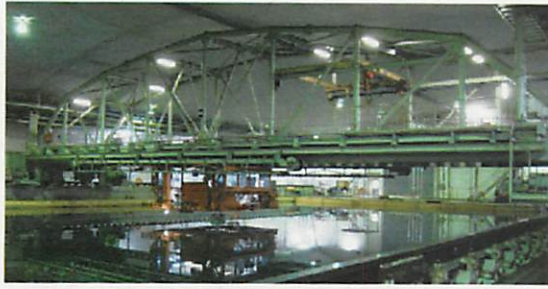
Fig. 2 View from forward of the subject ship fitted on the turntable during the CMT
