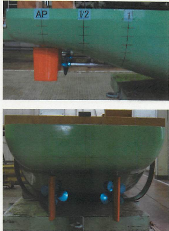
Fig. 1 Side view and stern view of the twin-propeller twin-rudder system for the subject ship
