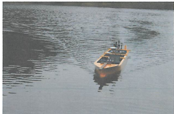
factor. Figure 2 Free model test in the manoeuvring pond of Osaka University
