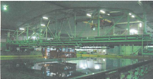
Figure 2 View from forward of a model ship fitted on the turntable during the CMT
