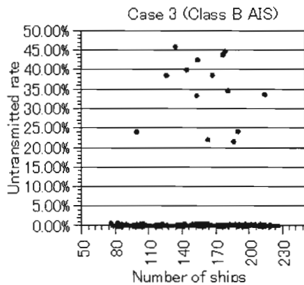
Fig. 9 Relation between un-transmitted rate and number of AIS equipped ships reachable from a specified ship equipped Class B AIS (Case3)
