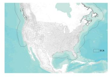
Note: Figure shows the regulated area for the North American Emission Control Area. Low sulfur fuel was required within the outlined boundary.
