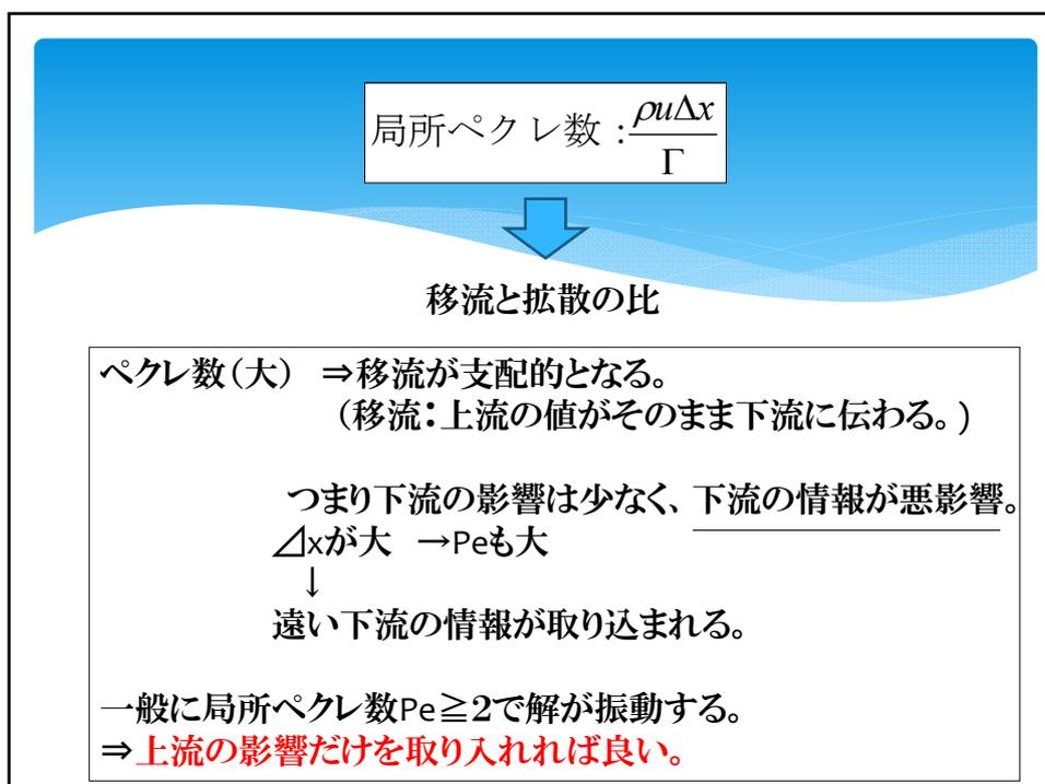
$\varphi_e = \varphi_P, \varphi_w = \varphi_W (u > 0 \Rightarrow Pe > 0)$  : 風上化
