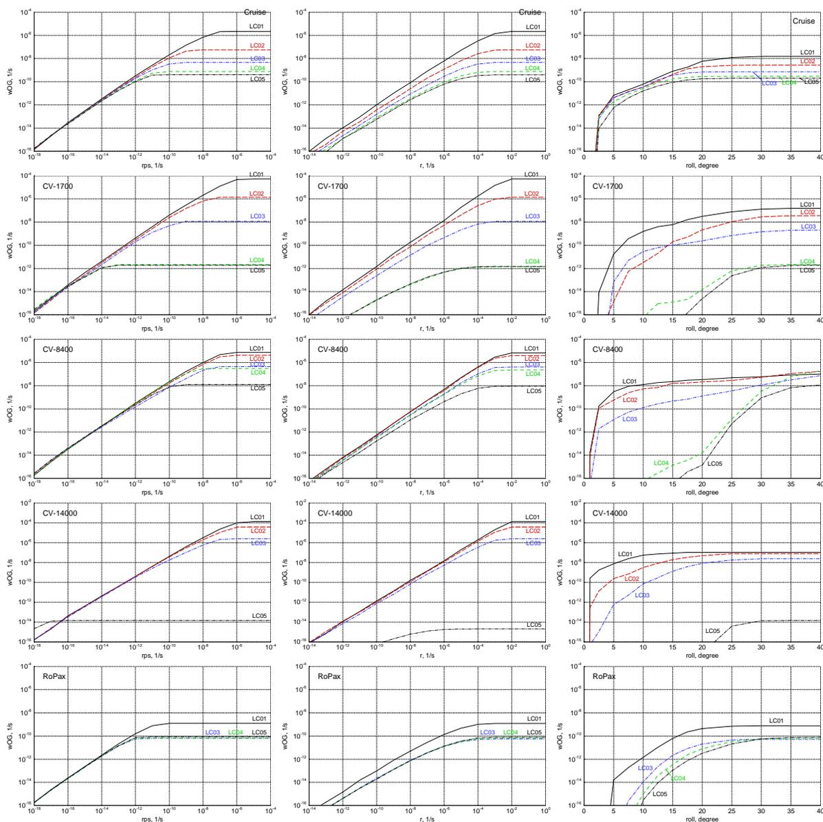
Figure 12. Long-term stability failure rate  $w_{OG}$  (averaged over all forward speeds) vs. short-term  $r_{ps}$ - (left),  $r$ - (middle) and  $\varphi_{3h}$ - (right) thresholds for different ships (rows) and loading conditions (different lines)
