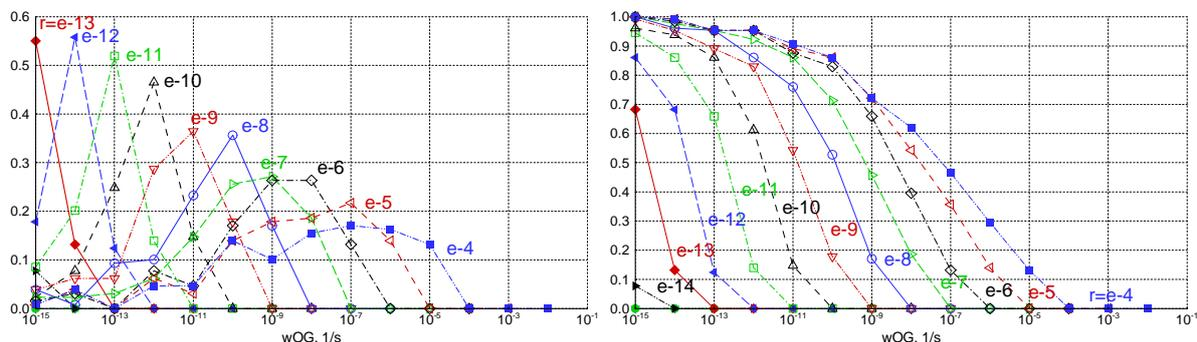
Figure 9. Left: histograms (number of ships, loading conditions and forward speeds normalized on 1) having long-term safety level  $w_{OG}$ , 1/s (x axis) for various  $r$ -threshold values (indicated in plot). Right: cumulative distributions derived from these histograms.
