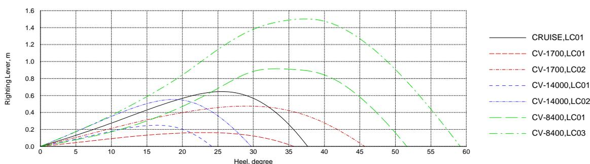
Figure 1. Calm-water righting lever curves for typical loading conditions with low GM
