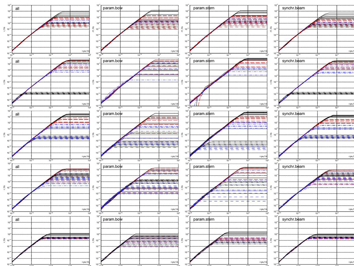
Figure 6. Average rate of stability failures  $w_{OG}$  (from left to right: all failure modes, parametric roll in bow waves, parametric roll in stern waves and synchronous roll) depending on  $r p_s$ -threshold for (from top to bottom) cruise vessel, CV 14000 TEU, CV 1700 TEU, CV 8400 TEU and RoPax; types and colours of lines differentiate loading conditions, lines of the same type and colour correspond to various forward speeds for same loading condition
