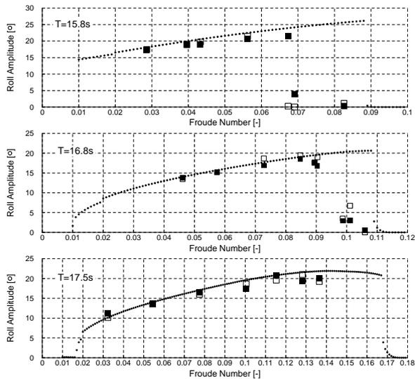
Figure 24. Measured (□,■) and computed (.) roll amplitude (y axis) in regular head waves vs. Fr (x axis) and wave period (one wave period per plot)
