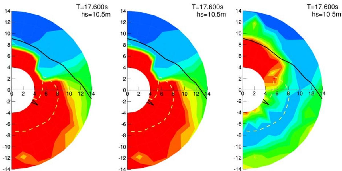
Figure 27. Colour plot of mean 3 hour maximum roll amplitude depending on forward speed (m/s, radial coordinate) and wave direction (circumferential coordinate, head waves at the top) for 8400 TEU container ship in loading conditions (from left to right) LC01, LC02 and LC03 together with line of maximum attainable speed (black solid line) and maximum available steering effort (yellow dashed line)
