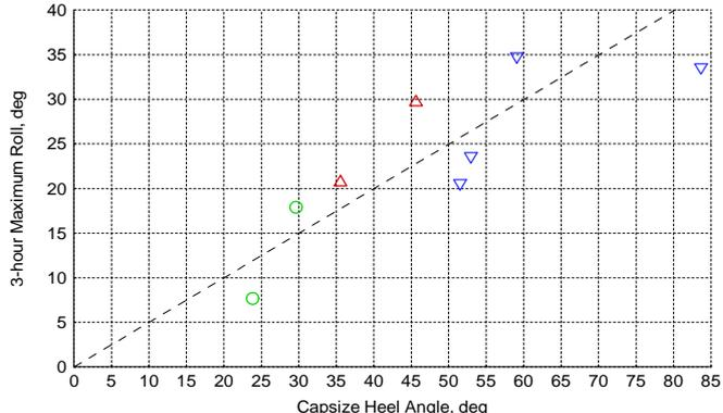
Figure 14.  $\phi_{3h}$ -threshold vs. calm-water capsizing heel angle
