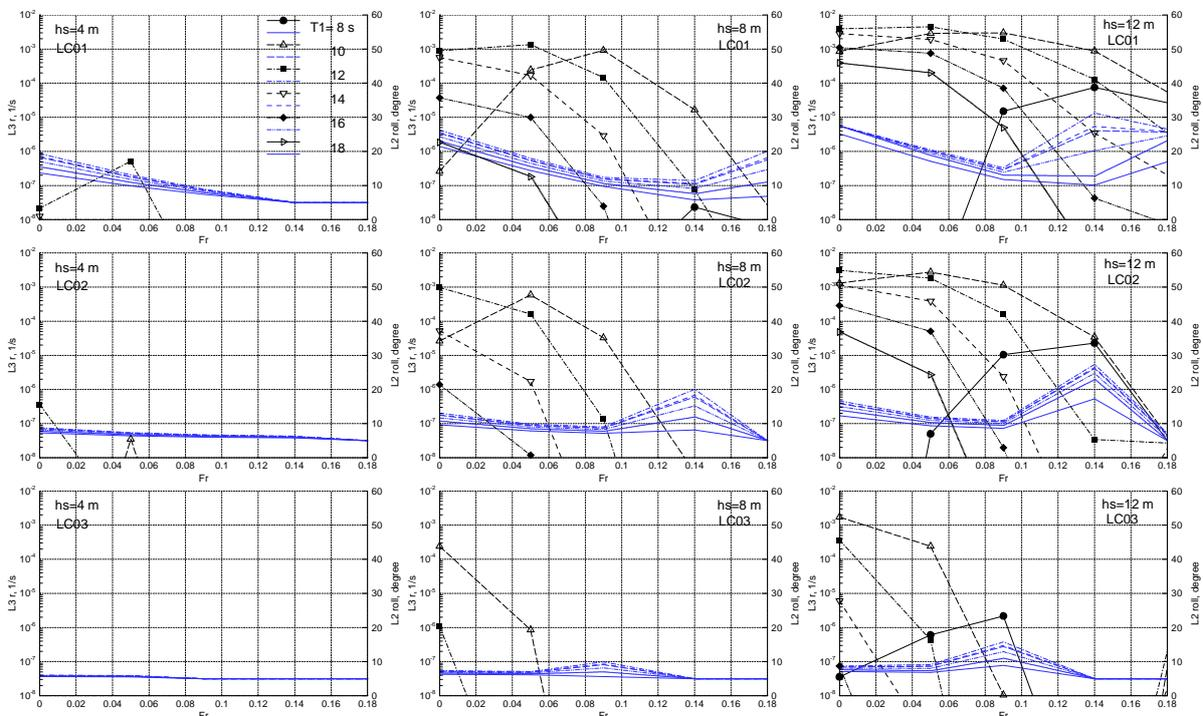
Figure 22. Failure rate due to parametric roll in following waves (left y axis, black lines with symbols) and roll amplitude from check 2 of level 2 PR criterion (right y axis, blue lines without symbols) vs. Fr (x axis) for 8400 TEU container ship in three loading conditions (each row corresponds to one loading condition) at significant wave height of (from left to right) 4, 8 and 12 m; different lines correspond to different wave periods
