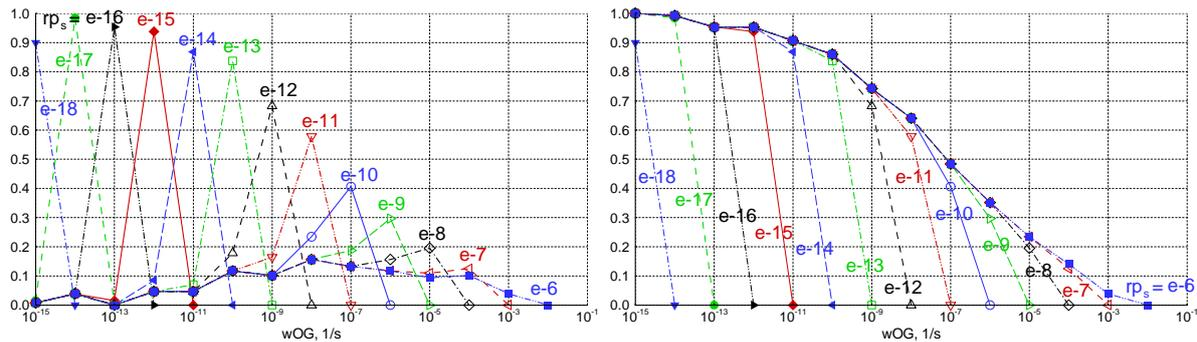
Figure 8. Left: histograms (number of ships, loading conditions and forward speeds normalized on 1) having long-term safety level  $w_{OG}$ , 1/s (x axis) for various  $rp_s$ -threshold values (indicated in plot). Right: cumulative distributions derived from these histograms.
