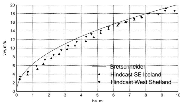
Figure 2. Theoretical relationship between wind speed (y axis) and wave height (x axis), solid line, in comparison with hindcast data for two locations in North Atlantic
