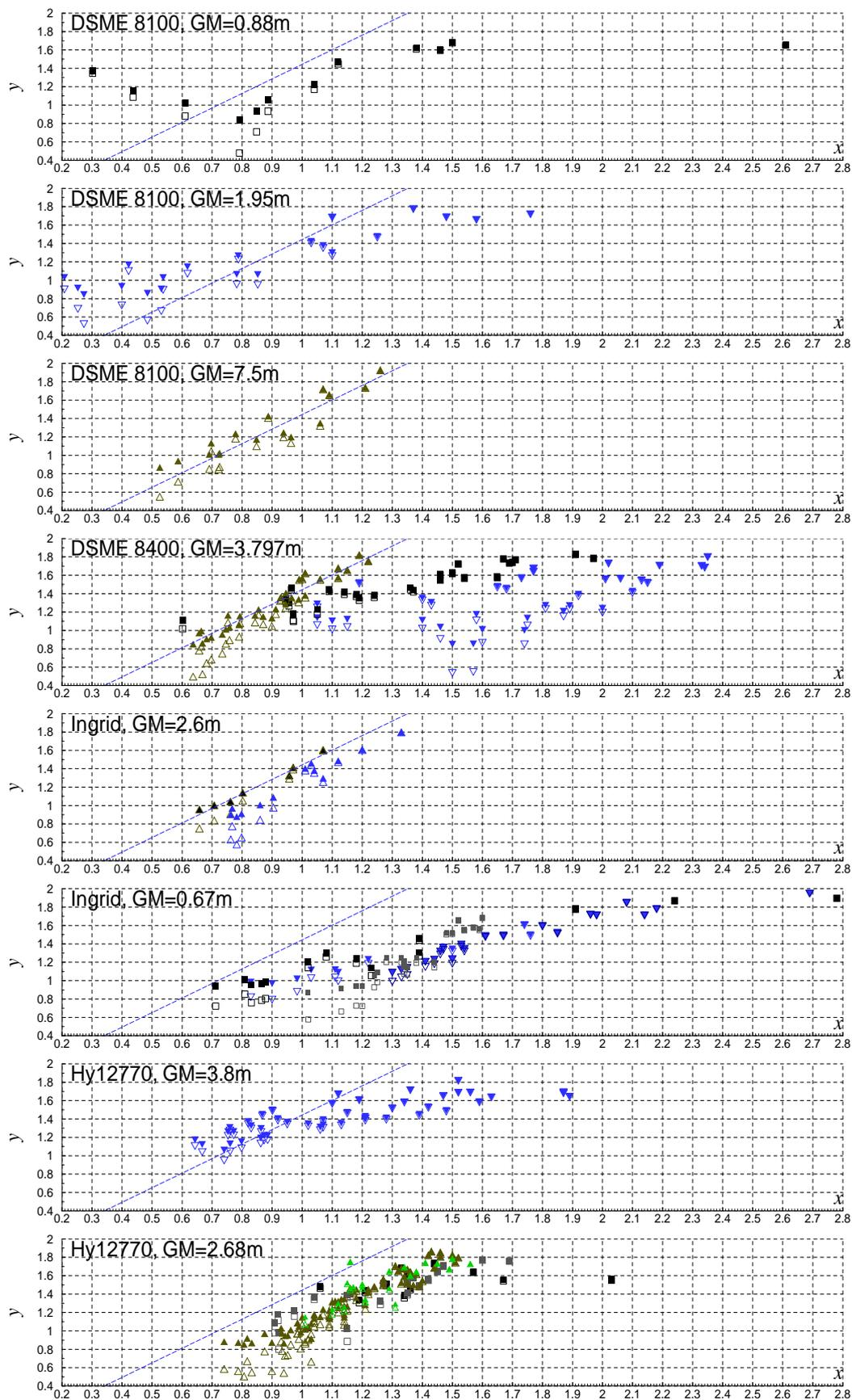
Figure 15.  $\ln(-\ln r)$  vs.  $\ln\{(\varphi_{3h} - \bar{\varphi})/\sigma_{\varphi}\}$  for parametric roll in stern-quartering (■, □) and bow (▼, ▽) waves and synchronous roll (▲, △); blue dashed lines show Rayleigh distribution
