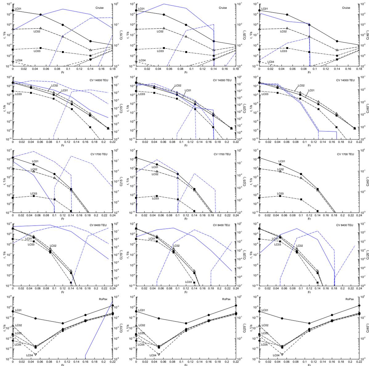
Figure 19. Parametric roll in head waves: direct assessment result  $w_{PR}^H$  (left y axis) and check 2 of level 2 result  $C_2^H$  (right axis) vs. Fr (x axis) for 15 (left), 25 (middle) and 40 (right) degree definition of stability failure for all loading conditions; each line corresponds to one loading condition: black lines with symbols refer to  $w_{PR}^H$ , same type blue lines without symbols to  $C_2^H$
