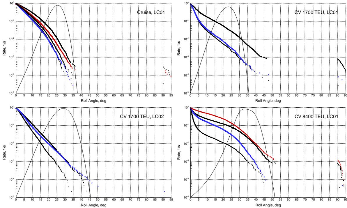
Figure 13. Cumulative distributions of exceedance rate vs. roll amplitude for (from left to right then top to bottom) cruise vessel in loading condition LC01 (examples of parametric roll in head and following waves and synchronous roll in beam waves), 1700 TEU container ship in LC01 (parametric roll in head and following waves) and LC02 (synchronous roll in beam waves) and 8400 TEU container ship in LC01 (parametric roll in head and following waves)
