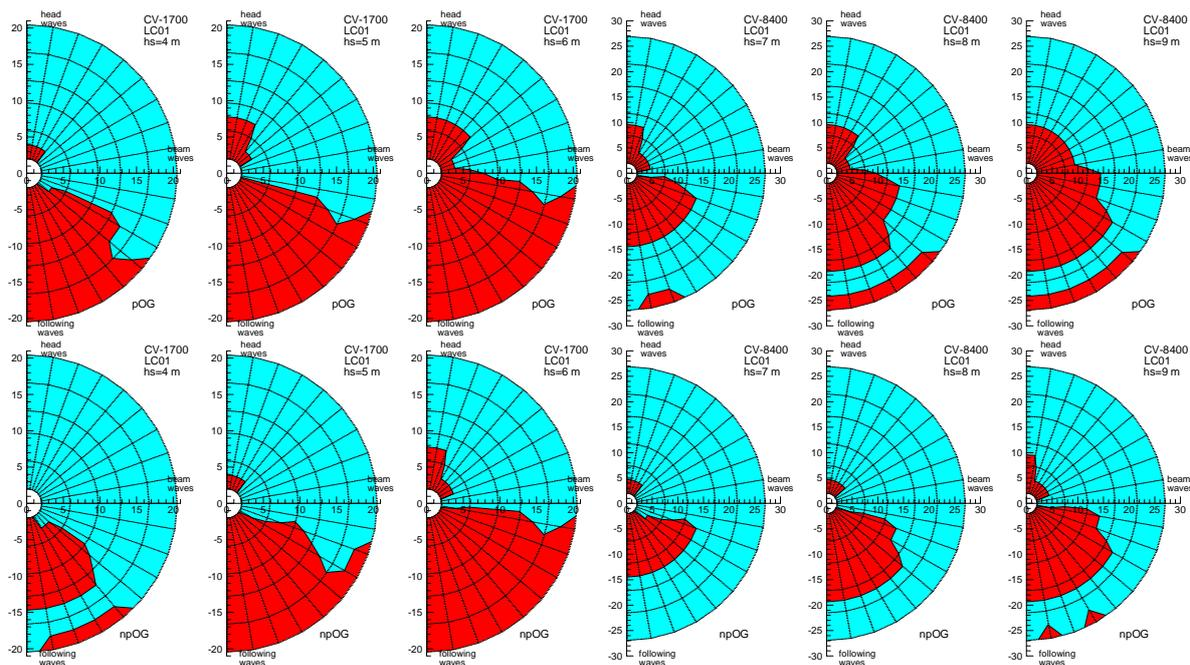
Figure 18. Examples of probabilistic (top) and non-probabilistic (bottom) operational guidance in axes ship speed (in knots, radial coordinate) – mean wave direction (circumferential coordinate) at different significant wave heights (columns) for 1700 TEU (three left columns) and 8400 TEU (three right columns) container ships
