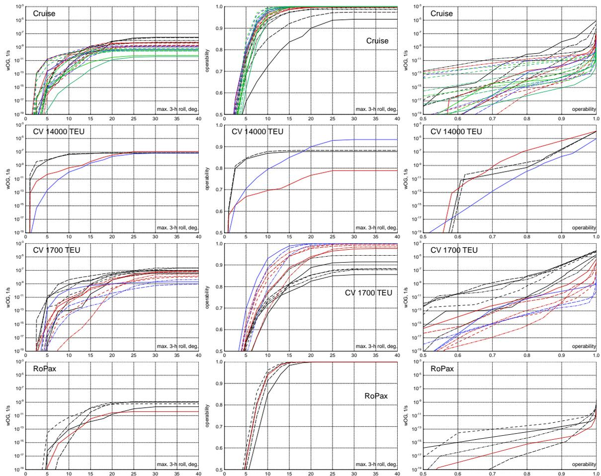
Figure 26. Left: mean long-term stability failure rate  $w_{OG}$  vs. threshold of mean 3-hour maximum roll amplitude; middle: operability vs. short-term threshold of mean 3-hour maximum roll amplitude; right: mean stability failure rate vs. operability for (from top to bottom) cruise vessel, CV 14000 TEU, CV 1700 TEU and RoPax; colours and line styles differentiate loading conditions and forward speeds, respectively
