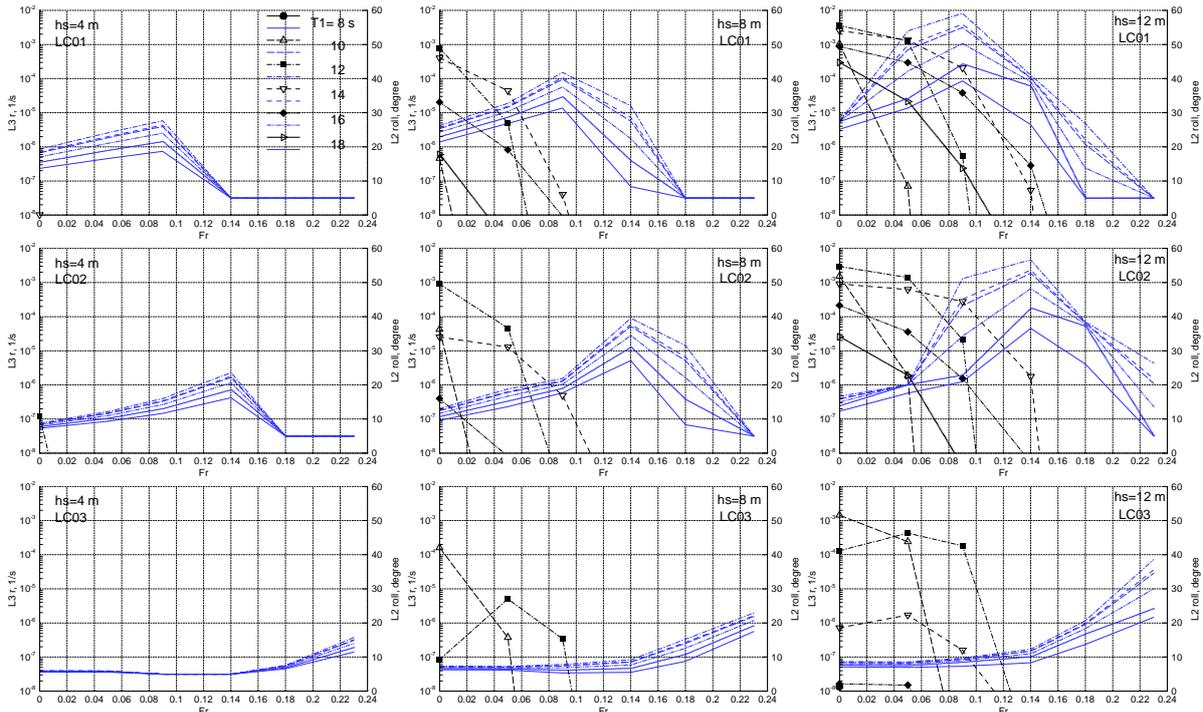
Figure 21. Failure rate due to parametric roll in head waves (left y axis, black lines with symbols) and roll amplitude from check 2 of level 2 PR criterion (right y axis, blue lines without symbols) vs. Fr (x axis) for 8400 TEU container ship in three loading conditions (each row corresponds to one loading condition) at significant wave height of (from left to right) 4, 8 and 12 m; different lines correspond to different wave periods
