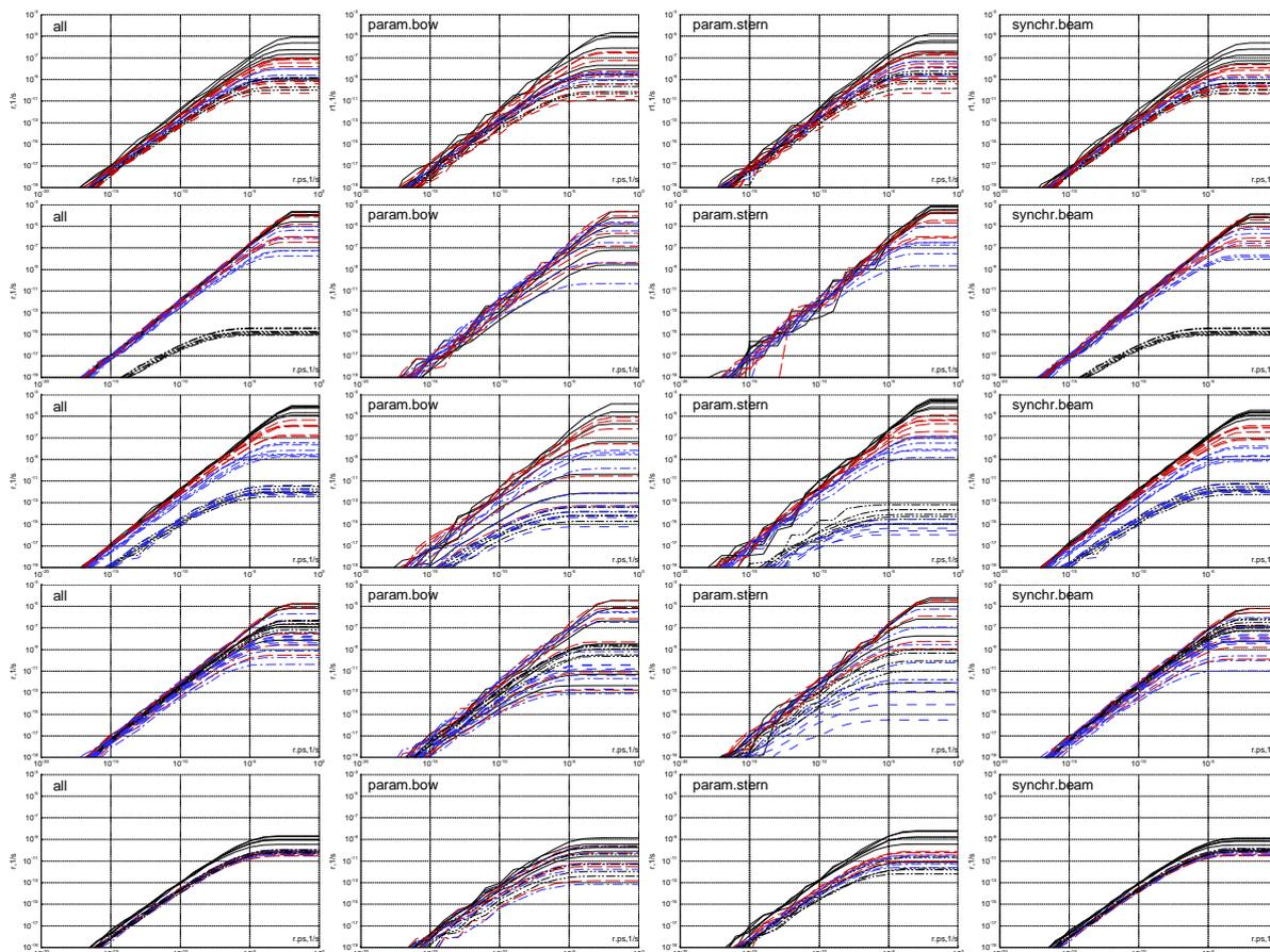
Figure 7. Average rate of stability failures  $w_{OG}$  (from left to right: all failure modes, parametric roll in bow waves, parametric roll in stern waves and synchronous roll) depending on  $r$ -threshold for (from top to bottom) cruise vessel, CV 14000 TEU, CV 1700 TEU, CV 8400 TEU and RoPax; types and colours of lines differentiate loading conditions, lines of the same type and colour correspond to various forward speeds for same loading condition
