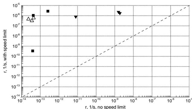
Figure 28. Rate of parametric roll stability failures in head waves considering (y axis) and not considering (x axis) attainable forward speed for three container ships (different symbols) in three loading conditions each
