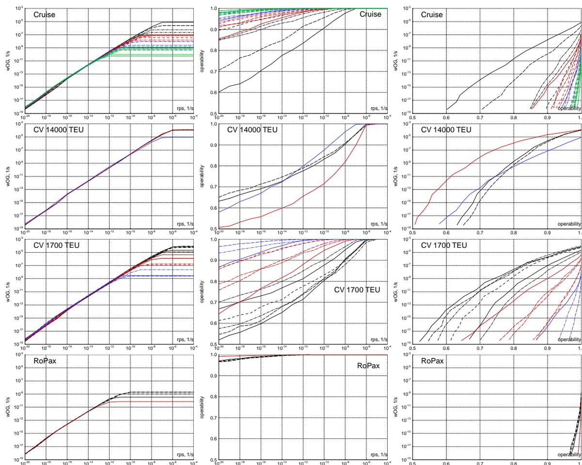
Figure 25. Left: mean long-term stability failure rate  $w_{OG}$  vs.  $rps$ -threshold, middle: operability vs.  $rps$ -threshold, right: mean stability failure rate vs. operability for (from top to bottom) cruise vessel, CV 14000 TEU, CV 1700 TEU and RoPax; curves of the same colour refer to the same loading condition, curves of the same style refer to the same forward speed
