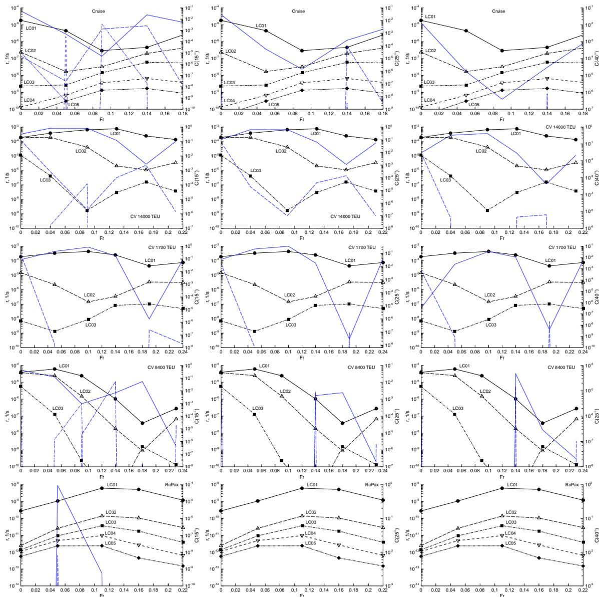
Figure 20. Parametric roll in following waves: direct assessment result  $w_{PR}^F$  (left y axis) and check 2 of level 2 result  $C_2^F$  (right axis) vs. Fr (x axis) for 15 (left), 25 (middle) and 40 (right) degree definition of stability failure for all loading conditions; each line corresponds to one loading condition: black lines with symbols refer to  $w_{PR}^F$ , same type blue lines without symbols to  $C_2^F$
