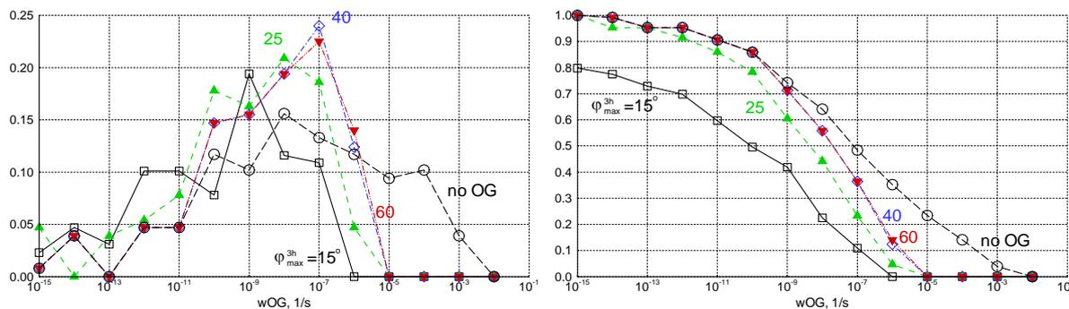
Figure 11. Left: histograms of total number of ships, loading conditions and forward speeds (normed on 1) having long-term safety level  $w_{OG}$ , 1/s (x axis) for various values (indicated in plot) of threshold of mean 3 hour maximum roll amplitude. Right: corresponding cumulative distributions.
