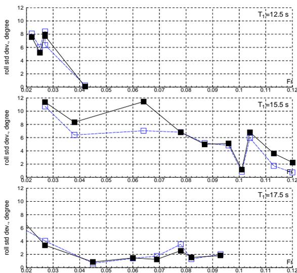
Figure 23. Measured (■) and computed (□) RMS of roll angle (y axis) in irregular head waves vs. Fr (x axis) and wave period (one wave period per plot)
