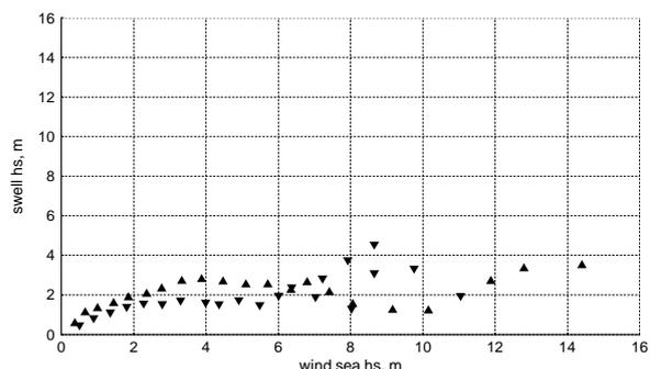
Figure 3. Significant wave height of swell (y axis) plotted vs. significant wave height of wind sea (x axis) for hindcast data shown in Figure 2
