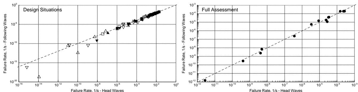
Figure 12. Stability failure rate due to parametric resonance in design situations at zero forward speed (left, symbols differentiate sea state probability density) and in full probabilistic assessment at zero forward speed (right) in following (y axis) vs. head (x axis) waves for all ships and loading conditions
