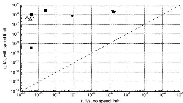
Figure 23. Rate of parametric roll stability failures in head waves considering (y axis) and not considering (x axis) attainable forward speed for three container ships (different symbols) in three loading conditions each
