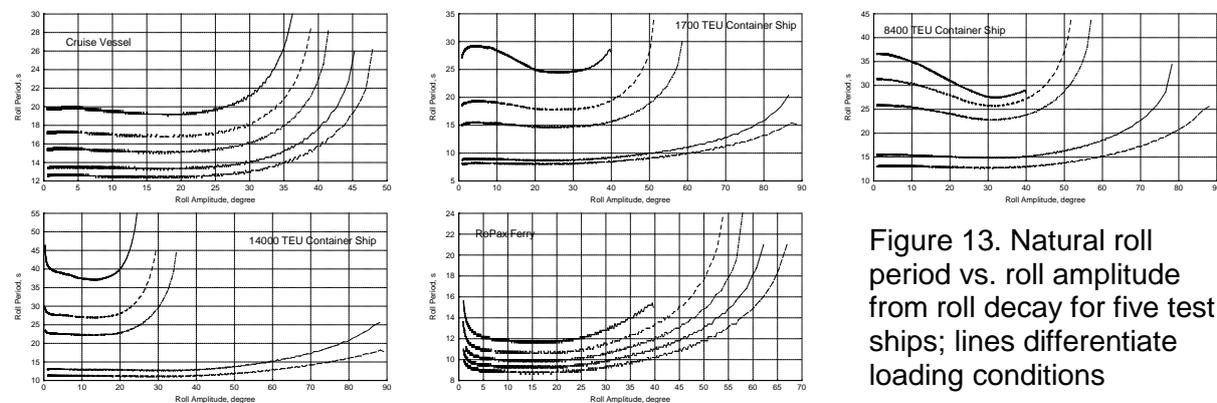
Figure 13. Natural roll period vs. roll amplitude from roll decay for five test ships; lines differentiate loading conditions
