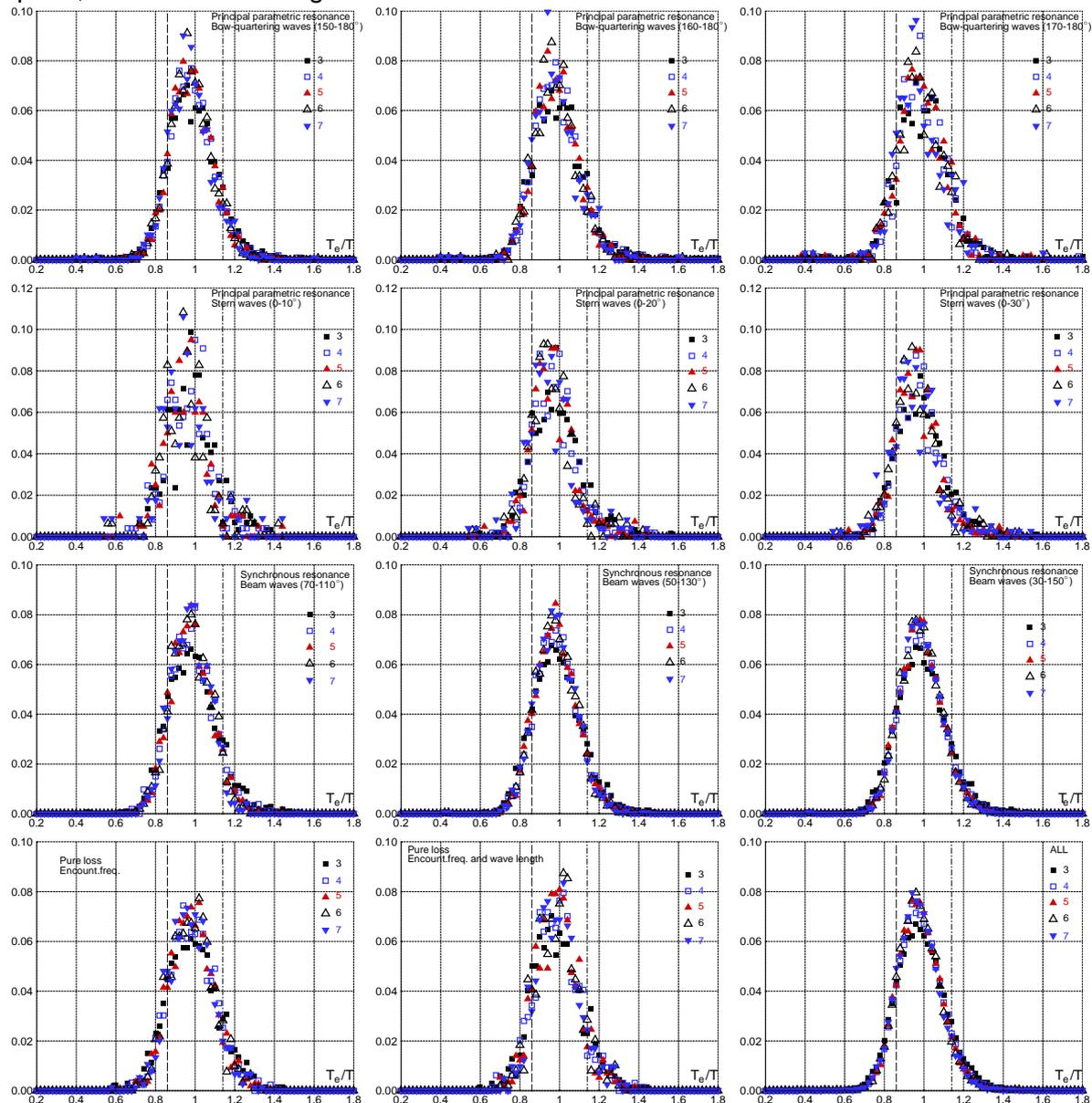
Figure 3. Histogram (number of cases normed on 1) of ratio  $T_{extr}/T$  and 95%-confidence interval of directly computed  $T$  (vertical lines) for (from top to bottom) parametric roll in bow waves, parametric roll in stern waves, synchronous roll in beam waves, pure loss of stability (bottom left and middle) and all cases together (bottom right); different symbols correspond to various number of points used in extrapolation over wave height
