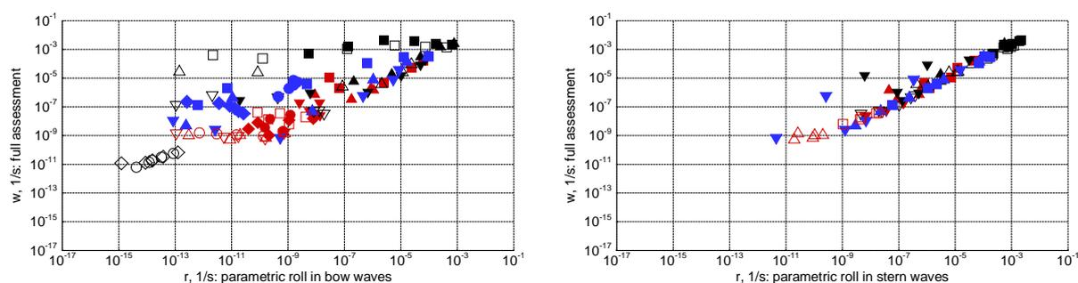
Figure 24. Contributions to mean long-term stability failure rate  $w$  (1/s, y-axis) from principal parametric resonance in bow (left) and stern (right) waves (1/s, x-axis); symbol types and colours differentiate ships and loading conditions
