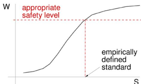
Figure 4. Idea of simplified safety criterion  $s$ ;  $w$  is the “true” safety measure, e.g. mean long-term probability of stability failure
