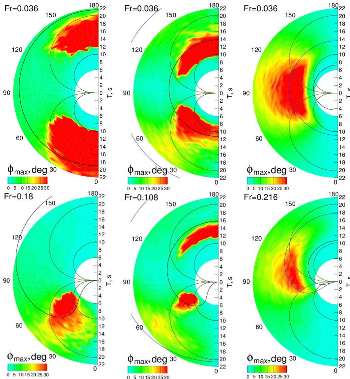
Figure 1. Colour plots of mean three-hour maximum roll amplitude depending on mean wave period (in s, radial coordinate) and mean wave direction (circumferential coordinate, waves from top, bottom and right correspond to 180, 0 and 90 degree, respectively) for principal parametric resonance at low (left) and medium (middle) GM and synchronous roll at high GM (right) at low (top) and high (bottom) forward speed
