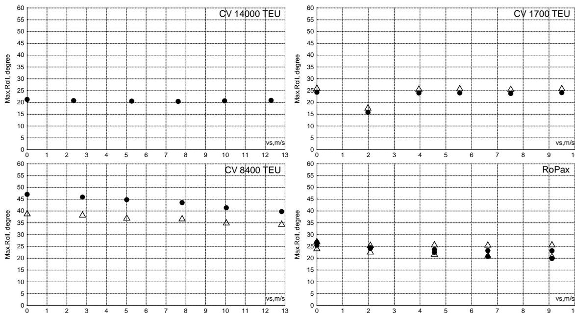
Figure 21. Mean 3-hour maximum roll amplitude due to synchronous roll in beam waves in sea states with  $f_s=10^{-5} \text{ (m}\cdot\text{s)}^{-1}$  vs. forward speed; each plot corresponds to one ship; different symbols correspond to different loading conditions
