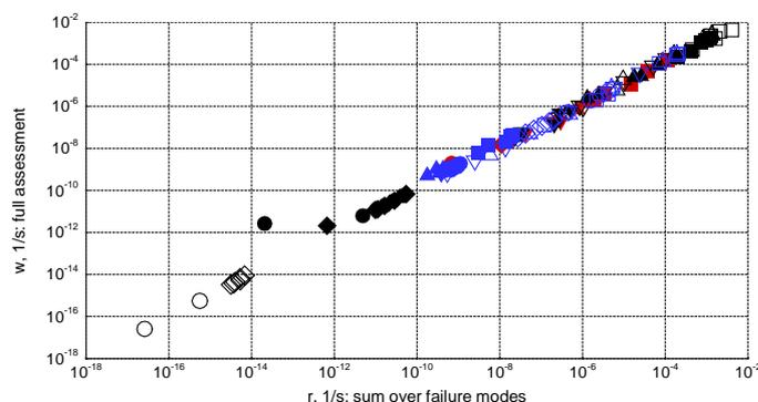
Figure 2. Total stability failure rate in all wave directions vs. sum of stability failure rates due to parametric roll in bow and stern waves and synchronous roll in beam waves; symbol type and colour differentiate ships and loading conditions
