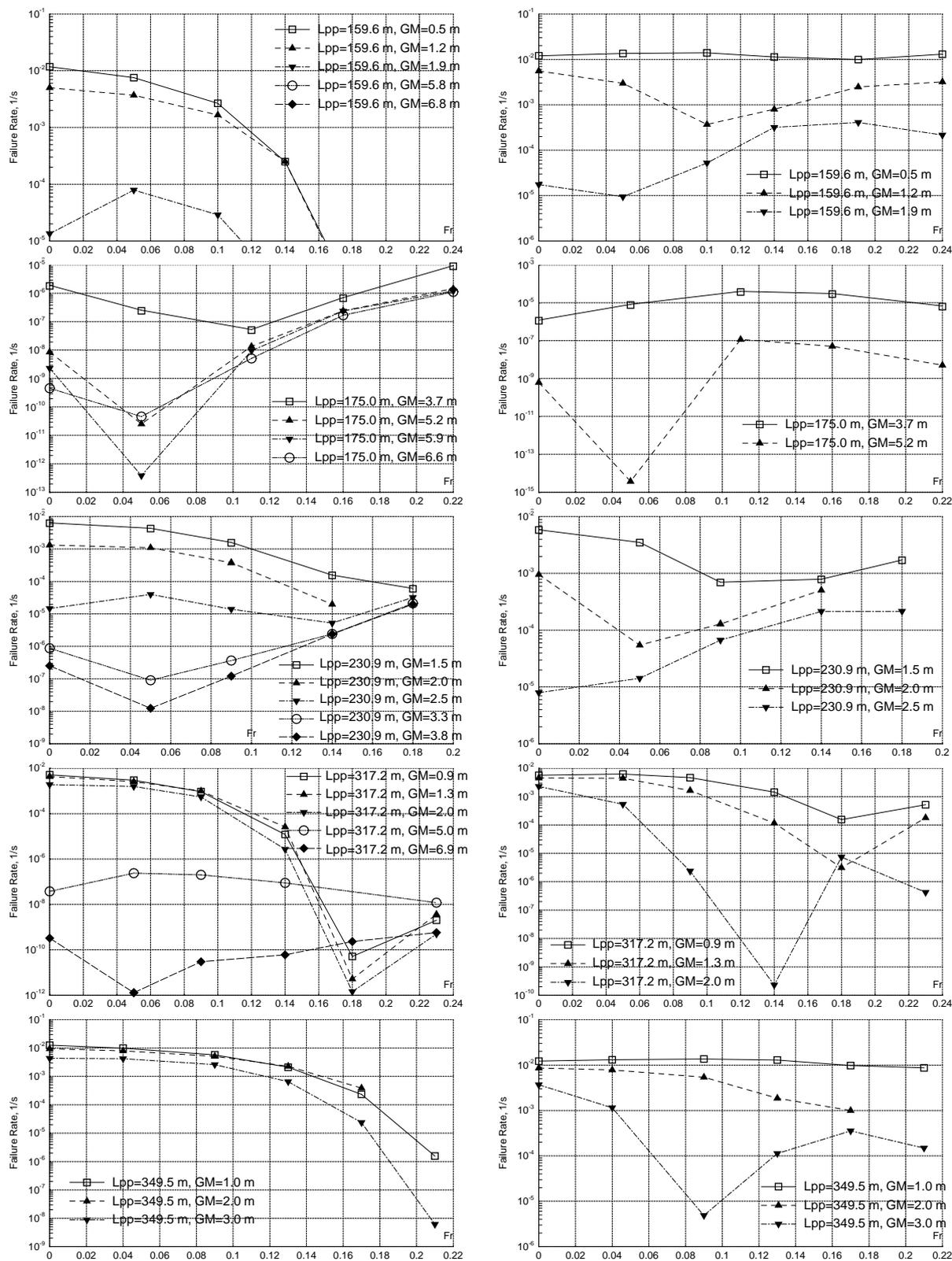
Figure 11. Maximum (over all wave periods) mean short-term stability failure rate, 1/s, at wave height corresponding to sea state probability density  $f_s=10^{-5}$  (in  $(m \cdot s)^{-1}$ , y axis) vs. Froude number (x axis) in head (left) and following (right) waves for (from top to bottom) 1700 TEU container ship, RoPax, cruise vessel and 8400 and 14000 TEU container ships; each line corresponds to one loading condition
