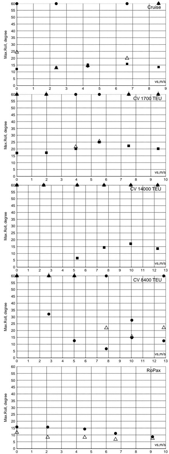
Figure 20. Mean 3-hour maximum roll amplitude due to parametric roll in following waves in sea states with  $f_s=10^{-5} \text{ (m}\cdot\text{s)}^{-1}$  vs. forward speed. Each plot corresponds to one ship; different symbols correspond to different loading conditions.
