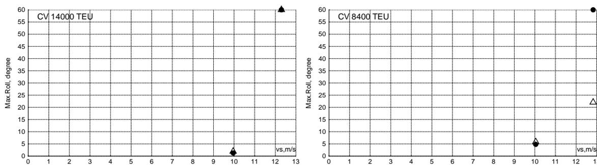
Figure 22. Mean 3-hour maximum roll amplitude due to pure loss of stability in following waves in sea states with  $f_s=10^{-5} \text{ (m}\cdot\text{s)}^{-1}$  vs. forward speed. Each plot corresponds to one ship; different symbols correspond to different loading conditions.
