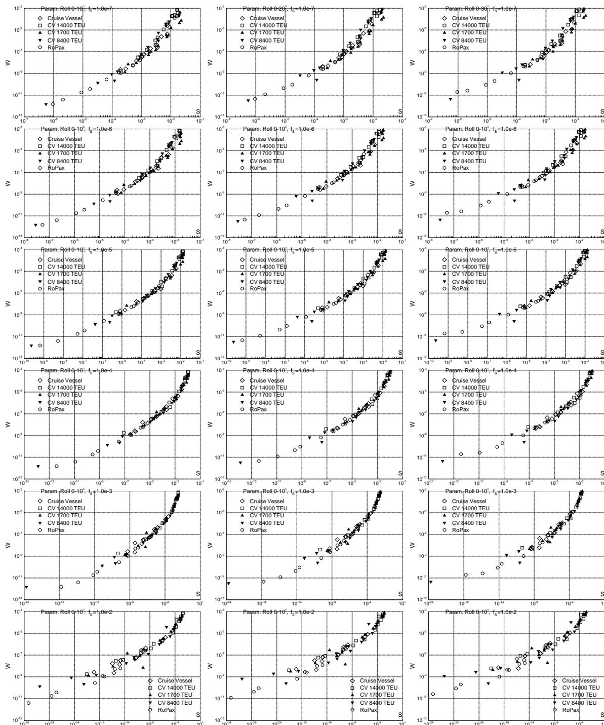
Figure 7. Dependencies  $w(s)$  for design situations for parametric roll in stern waves: mean long-term stability failure rate  $w(\text{ship}, \text{LC}, v_s)$ ,  $1/s$ , y axis, in wave directions 0 to 10 degree (left), 0 to 20 degree (middle) and 0 to 30 degree (right) vs. simplified criterion,  $1/s$ , x axis – short-term mean stability failure rate in following waves, maximum over design sea states
