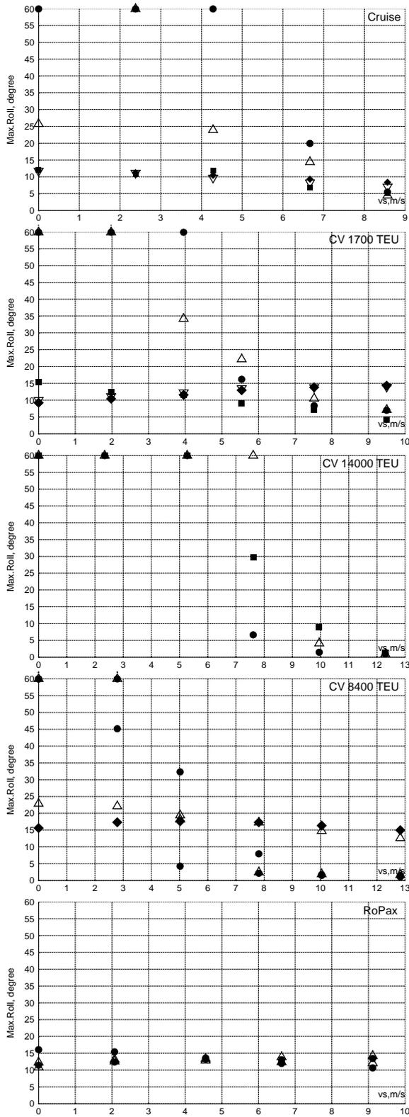
Figure 19. Mean 3-hour maximum roll amplitude due to parametric roll in head waves in sea states with  $f_s=10^{-5} \text{ (m}\cdot\text{s)}^{-1}$  vs. forward speed. Each plot corresponds to one ship; different symbols correspond to different loading conditions.
