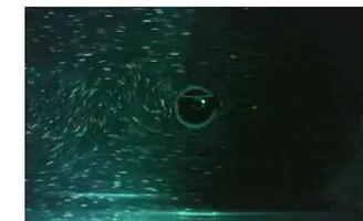
Visualization of the flow field around the circular cylinder supported by spring at both end
