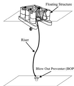
Example of long flexible pipe (riser pipe)
