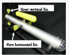
Biomimetic Underwater Robot equipped with 4 mechanical pectoral fins (PLATYPUS)
