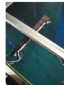
Forced oscillation experiment using a flexible pipe model (6.5[m])
