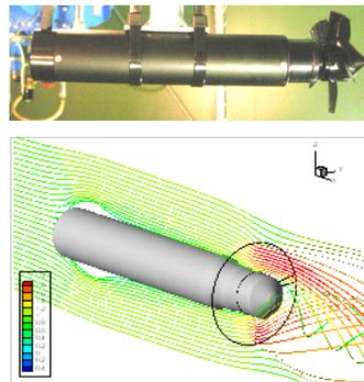
Thruster for underwater vehicle (upper) and Computational result of flow field around the thruster (lower)
