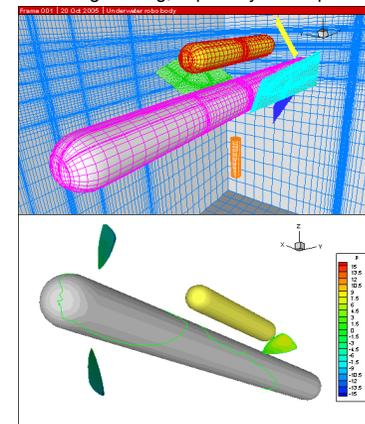
Computation around a underwater vehicle with mechanical pectoral fins "PLATYPUS"
