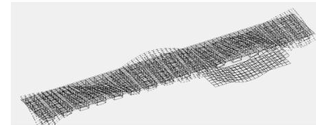
Response of VLFS consisting of semi-submersible type runway and pontoon type apron.
