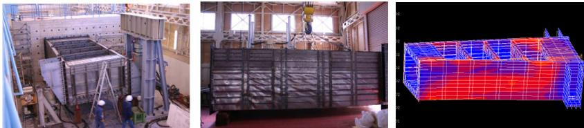
Experimental collapse analysis by using a scaled model and computer simulation (L=8m, B=3m, D=2m)
