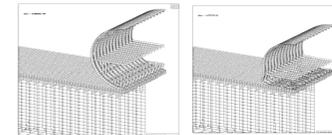
Simulation of belly-landing of an airplane to VLFS
